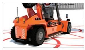
Two antennas have been installed at the back covering steer area of the reachstacker.
